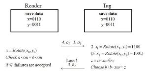
Figure 2: The asynchronous flaw in HB-MP scheme
