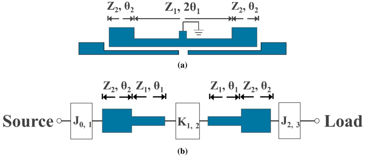
Figure 2. (a) 2-order filter structure and (b) alternative J and K inverters.
