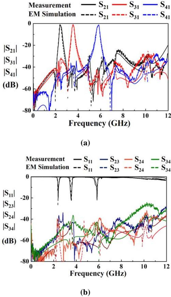
Figure 7. Simulated and measured results of (a) return loss, (b) insertion loss and in-band isolation of the proposed triplexer. The dimensions are  $L_1 = 40$ ,  $L_2 = 12.1$ ,  $L_3 = 9.6$ ,  $S_4 = 0.3$ ,  $S_1 = 0.2$ ,  $S_2 = 0.2$ ,  $S_3 = 0.2$ ,  $W_1 = 0.5$ . (All are in mm).
