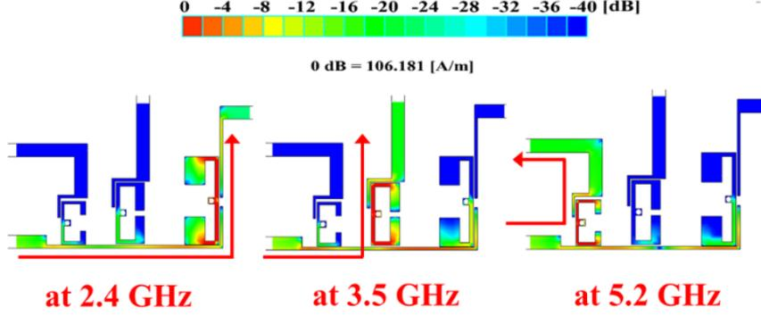
Figure 5. Current distribution of the proposed triplexer.
