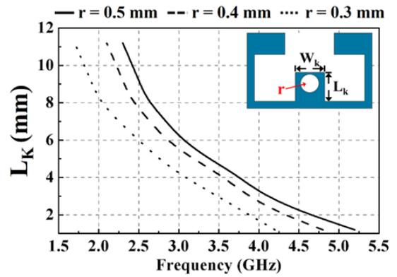
**Figure 5.** Relations between the short-circuited stub length  $L_K$  and size of via hole for passband frequencies tuning. ( $r$  indicates the radius of the via hole)
