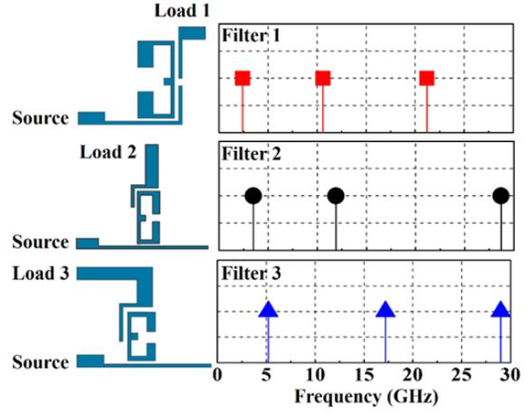
**Figure 4.** The distribution of fundamental and higher order resonant frequencies of the proposed SIRs for each channel.
