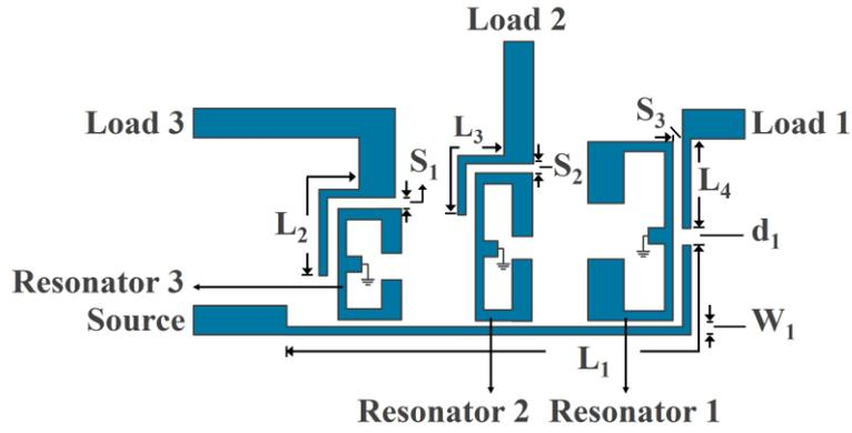
Figure 1. Configuration of the proposed triplexer. (Number 1, 2 and 3 indicate the index of bandpass filter in this work)
