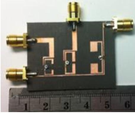
Figure 6. Photograph of the fabricated triplexer.
