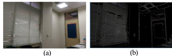
**Figure 23 The result of Canny edge detection**
