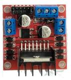
Figure 4. L298N motor drive board module
