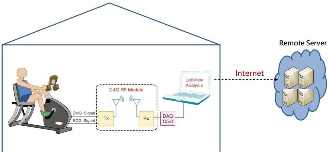
Figure 2. Portable wireless multiparameter system for the assessment of exercise-induced fatigue.
