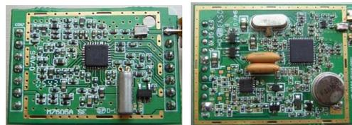
**Figure 6. B RW67RX-SA01 wireless transmission and reception module.**
