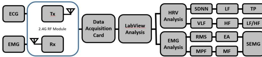
**Figure 3. Block diagram for the proposed measuring system.**
