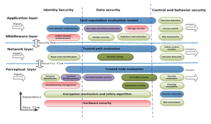
Fig. 3 A hierarchical security architecture.
