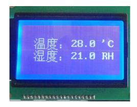
Figure 4: 12864 LCD Module
