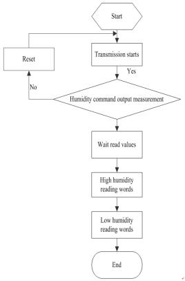
Figure 8: Program flow measuring temperature and humidity
