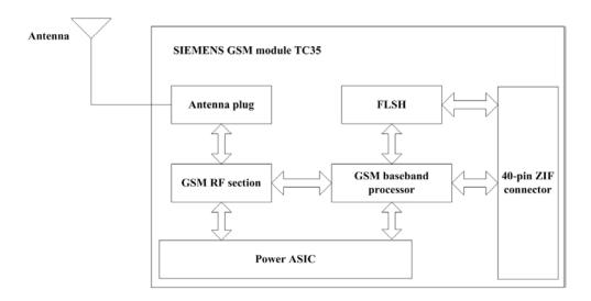
Figure 2: TC35i module structure diagram
