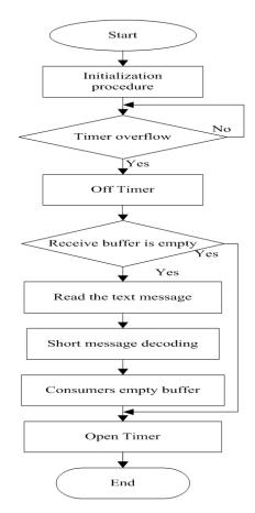
Figure 10: Receiving SMS program flow
