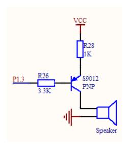
Figure 6: Transistor drive circuit buzzer sounds alarm
