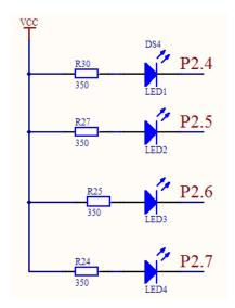
Figure 7: LED alarm circuit
