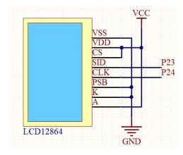
Figure 5: SCM and 12864 connection diagram
