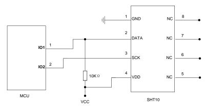
Figure 3: microprocessor hardware connection diagram with SHT10
