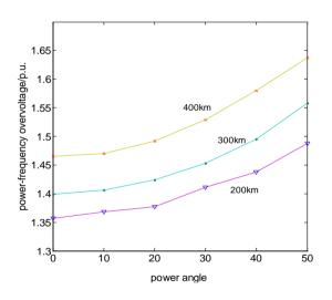
Figure 1: The influence of the power angle to power-frequency overvoltage
