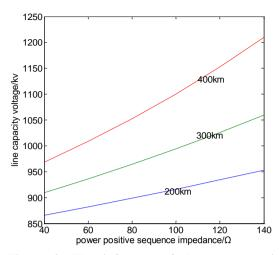
Figure 3: The influence of the power positive sequence impedance to line capacity voltage rise
