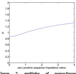
Figure 2: multiples of power-frequency overvoltage when Single-phase ground fault
