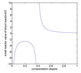
Figure 12: The relationship between small reactor value of shunt reactor and compensation degree
