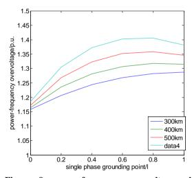
Figure 9: power-frequency overvoltage when single phase grounding at different point
