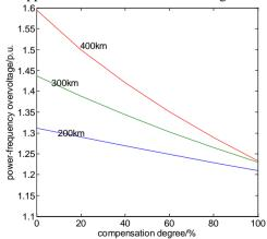
(a) power-frequency overvoltage when m end three-phase tripping
