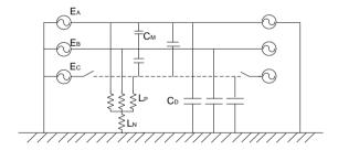
Figure 10: Schematic diagram of open-phaseoperation
