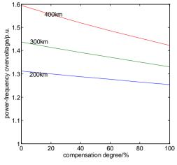
Figure 7: The influence of compensation degree to power-frequency overvoltage when HV shunt reactor at sending end of the line
