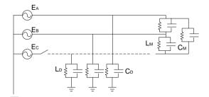
Figure 11: The equivalent figure of open-phase operation with high voltage shunt reactor
