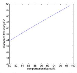
Figure 16: resonance frequency under different compensation degree
