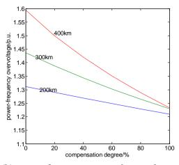
(b) power-frequency overvoltage when n end three-phase tripping
