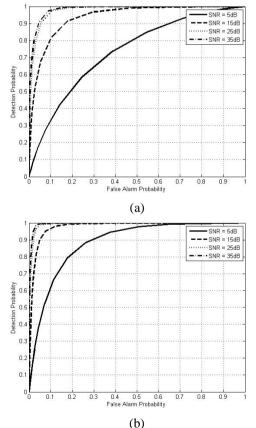
Figure 3: Receiver Operating Characteristic (ROC) curves of (a) KFLM and (b) CEM, in computer-simulated phantoms with different SNRs.
