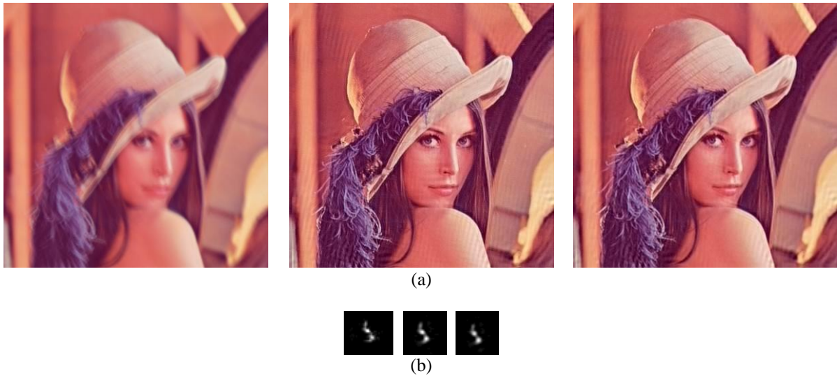
Figure 1: Deblurred result of “Lena”. (a) From left to right, images are input blurred image, result of Cho’s method and result of proposed method. (b) Corresponding PSF of (a). From left to right, ground truth, PSF of Cho’s method and PSF of proposed method. We can observe that ringing artifact on the face of Lena is removed.
