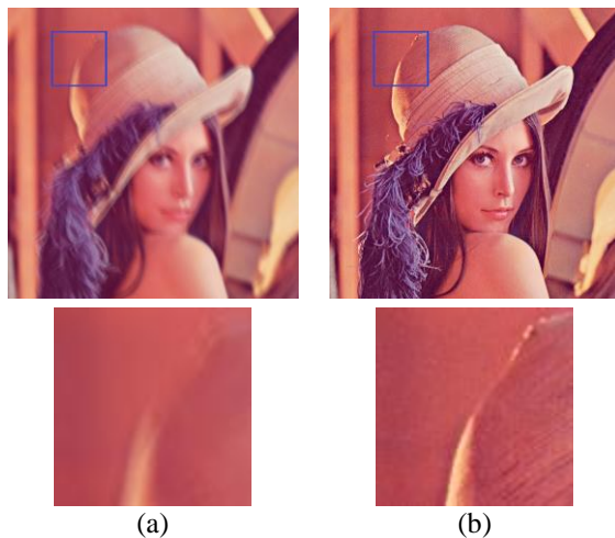
Figure 1: Example of local priors. (a) Blurred image. (b) Original unblurred image. The first row is full size images and the second row is the close-up views corresponding to the blue rectangle in the first row images. From this example, we can notice that smooth regions of the blue rectangle in blurred image are also smooth in original image. We use this information as local priors for image deblurring.
