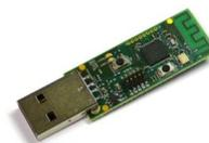
Figure 19: CC2531 USB Evaluation Module Kit
