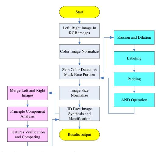
Figure 2: The flow chart of the 3D face rewcognition
