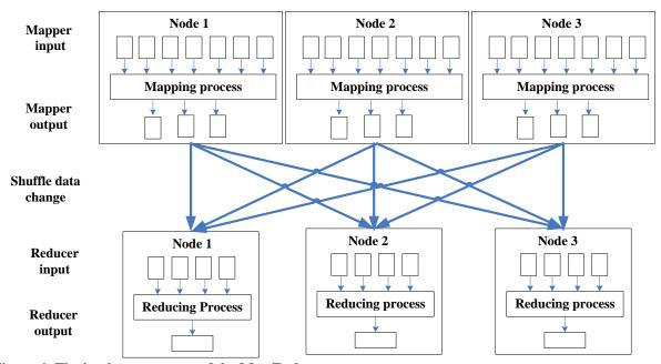
Figure 6: The implement system of the Map/Reduce stream
