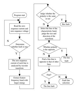
Figure 1: Flow diagram of selection line
