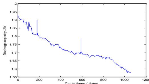
**Figure 7: The capacity attenuation of lithium-ion battery after denoising**
