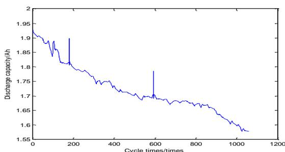
Figure 2: The capacity attenuation of the original test data for Lithium-ion battery
