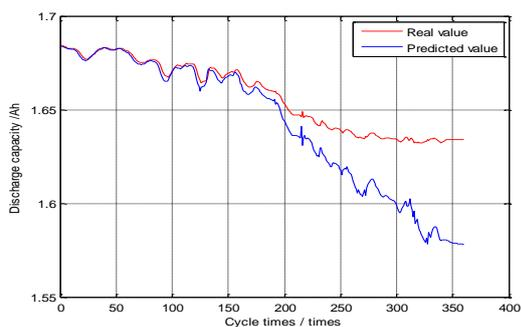
**Figure 9: The results of life prediction for Lithium-ion Battery**
