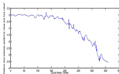
**Figure 10: The relative error between the predicted value and the real value of the lithium-ion battery life**
