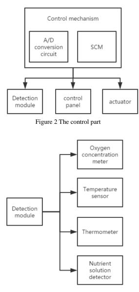
Figure 3 The detection module
