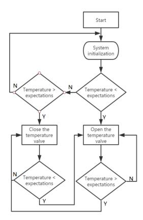
Figure 7 Temperaturecontrol flow chart
