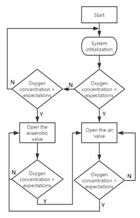
Figure 6 Oxygen concentration control flow chart
