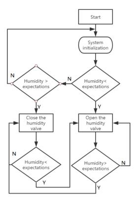
Figure 8 Humiditycontrol flow chart
