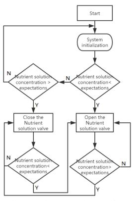
Figure 9 Nutrient concentrationcontrol flow chart
